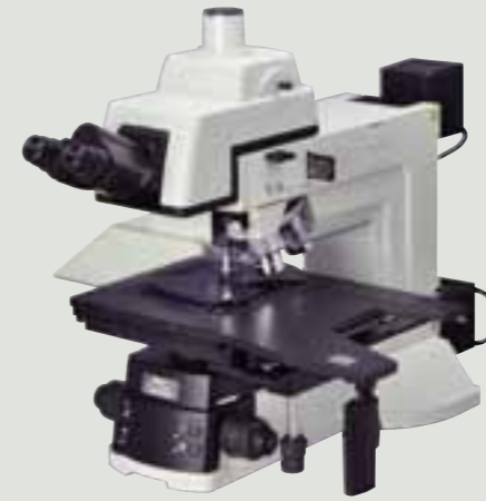
For ø200mm wafer/Episcopic illumination type ECLIPSE L200N
