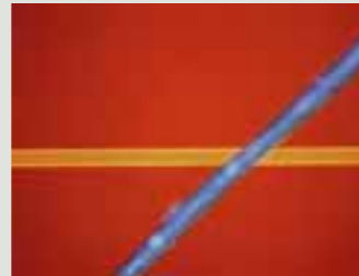
Epi-fluorescence observation of organic substance on wafer
