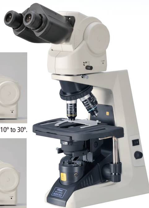
E200 configured with an ergonomic binocular tube.
